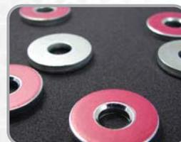
**Structural Adhesive Tape** Argent's patented Epoxy Washer System uses a thermosetting epoxy film to permanently adhere metal washers to automotive hinge assemblies. Primarily used for "doors-off" assembly, the Epoxy Washer System maintains door alignment for easy reattachment at the final stages of the assembly process. Our epoxy washers are conveniently supplied on trays. Please contact us for more information. U.S. Patent # 6669428
